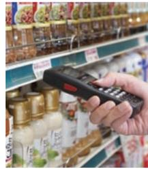
Scanning from a remote position is available as well as touch-scanning, which can easily read a barcode only by touching the reading window to it. Even novices can easily use it as they don't need to pay much attention to the scanning position.
