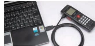
You can connect the terminal directly to a PC using a USB cable. Power supply from the USB terminal is available as well as high speed communication through the terminal, so you don't need to worry about the remaining battery charge.
